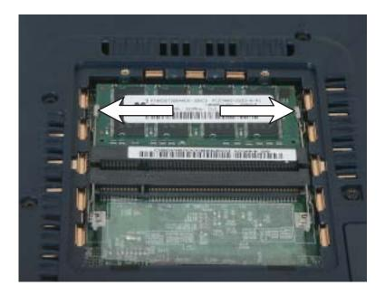
**7** Pull the memory module out of the slot.
